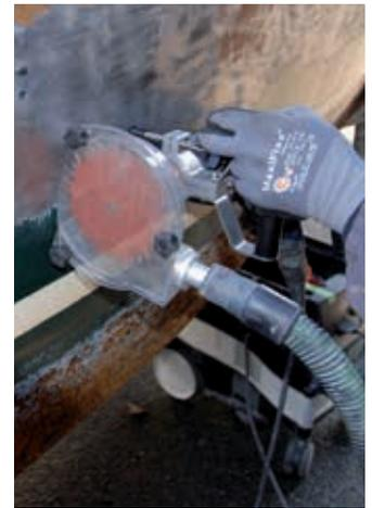
Removing paint with adjustable guide and dust cover
